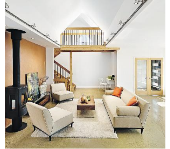
Above: Belgravia Green's concrete floor absorbs sunlight and recirculate it to heat the house. Right: A wood stove is used to pick up heating slack during the winter.
